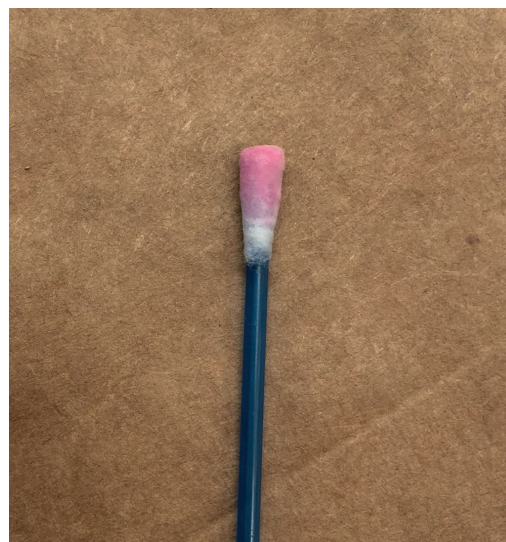
FIGURE 2: Nickel spot test with a strong positive result
