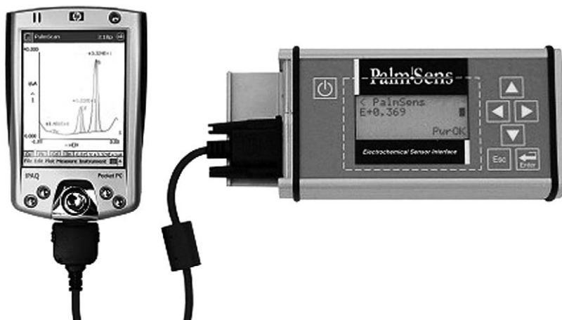
Fig. 29.1. Hand-held potentiostat by PalmSens used in all the optimization protocols described in the text.
