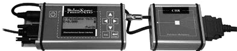
Fig. 29.3. The PalmSens hand-held potentiostat equipped with the dedicated multiplexer for eight-channel measurements.
