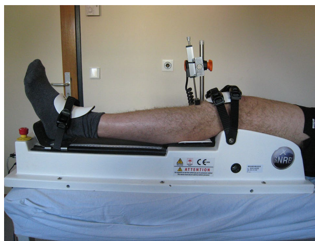
Fig. 1 Device used for the static anterior knee laxity measurements (GNRB ® )
