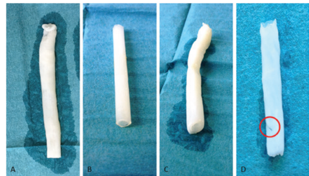
Figure 2: By high-speed rotation molding, 100-mm-long fibrin tubes were generated with an outer diameter of 7 mm (A). During dehydration, the tubes shrank to the diameter preset of the dilator inside (B). After 6 months of storage in dry air, all fibrin tubes were intact (C), whereas after 12 months, most of the tubes had fissures (indicated in D).
