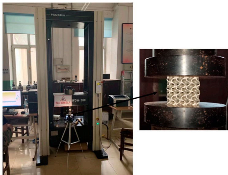
Figure 4. Universal mechanical testing machine and test process.
