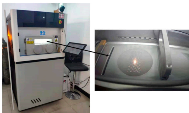
Figure 3. SLM printer and the printing process.
