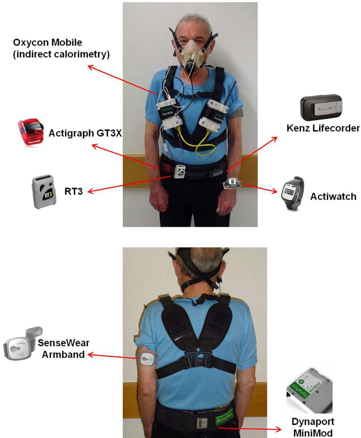
Figure 1. Location of attachment for the Oxycon Mobile and the six activity monitors. doi:10.1371/journal.pone.0039198.g001
