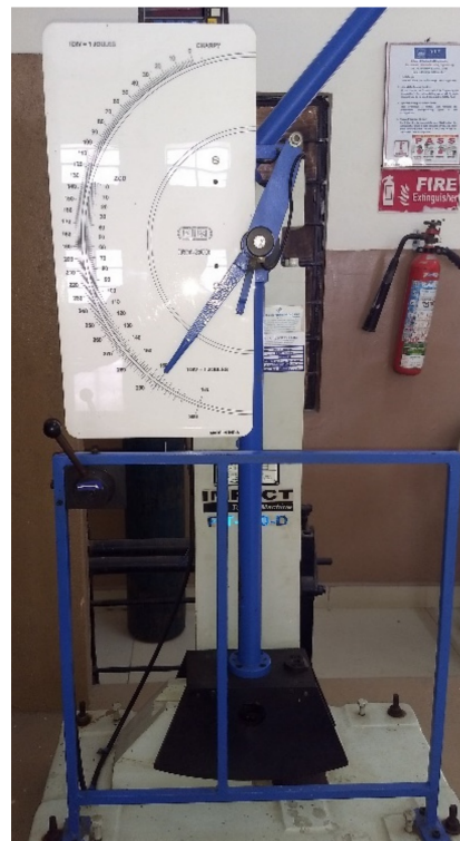
Figure 11. FIT-300-D model impact tester.
