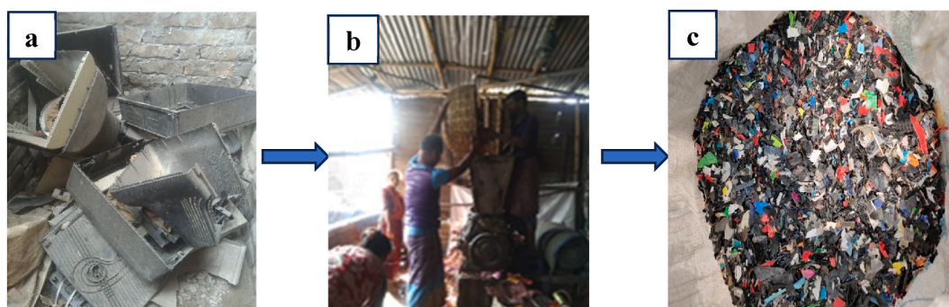
Fig. 1. The manufacturing process of PCA (a) collecting e-waste plastic (b) shredding or grinding (c) ground or crushed into little pieces.
