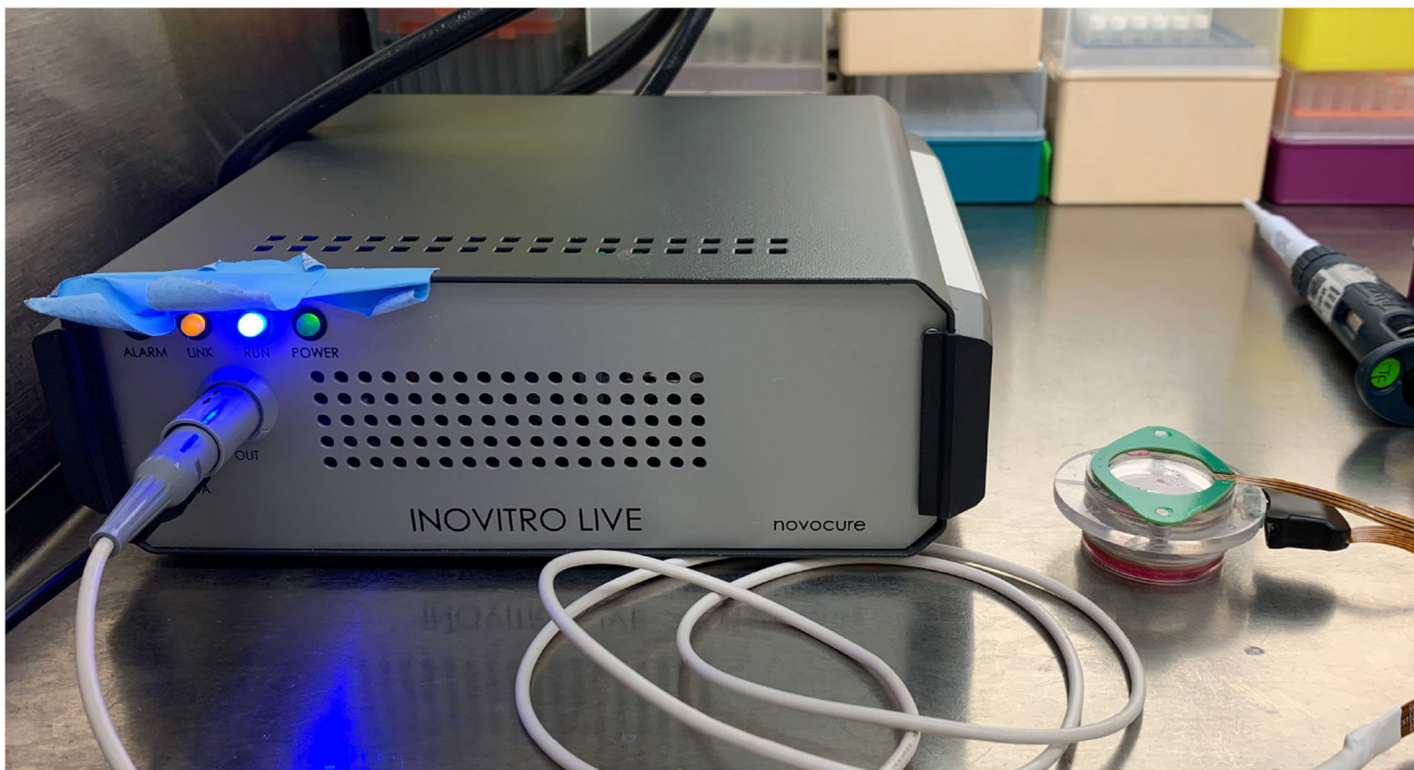
FIGURE 1 | A digital photograph of the inovitro live system. The inovitro live TTFields generator is shown on the left with the ceramic insert and the attached cover heating element visible on the right.
