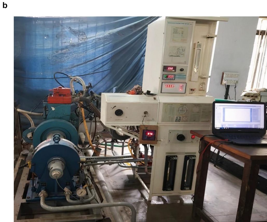
Figure 1. (a) Schematic of the test set-up. 1-Engine, 2-Dynamometer, 3-Computer, 4-Calorimeter, 5- Autogas -Cylinder, 6-Fuel tank, 7-Wet flame arrester, 8-Exhaust gas analyzer, 9-Flywheel, 10-Starter motor, 11-Manometer, 12-Fuel burette, 13-Air-box, 14-Water rotameters, 15-Load knob, 16-Open ECU (primary), 17-Gas ECU, 18-Battery, 19-Capacitor, 20-Throttle-body, 21-Sequential reducer, 22-Dry flame trap, 23-T7 display, 24-Inlet-manifold, 25-Exhaust manifold, 26-Spark-plug, 27-Water inlet (dynamometer), 28-Water inlet (engine), 29-Water outlet (dynamometer), 30-Water outlet (engine), 31-Water inlet (calorimeter), 32-Water outlet (calorimeter), C-Crank encoder, D-Crank Position Sensor, G-Pressure gauge, M-MAP Sensor, P-Pressure Transducer, R-Gas rotameter, S-Safety valve, T1-Thermocouple (inlet water, engine & dynamometer), T2-Thermocouple (outlet water, engine), T3-Thermocouple (inlet water, calorimeter), T4-Thermocouple (outlet water, calorimeter), T5-Thermocouple (exhaust gas inlet, calorimeter), T6-Thermocouple (exhaust gas outlet, calorimeter), T7-Thermocouple (exhaust gas, manifold), V- Autogas Supply valve. (b) Experimental test-rig.
