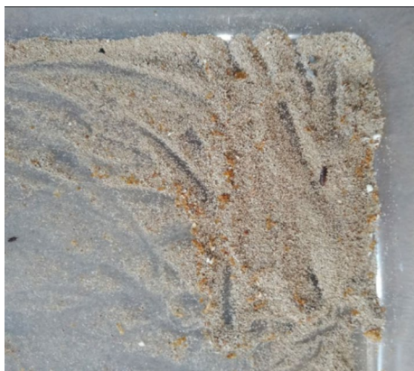
Fig. 3 Frass excreted by the Tenebrio molitor mealworms after being fed with polystyrene
