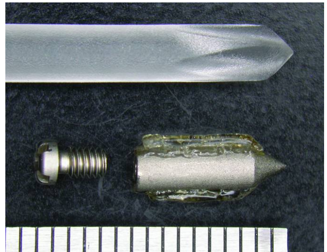
Fig. (2). Pictures of the implants. The pure PLA-pin (top) was fixed directly at the sonotrode, while an adaptor was used for the titanium-PLA pin (Ti-PLA)(bottom, above the millimeter scale). Polymer stripes were sintered at the titanium core.
