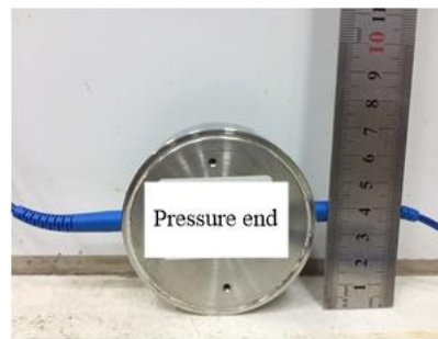
Figure 7. Pile top temperature self-compensating pressure sensor.
