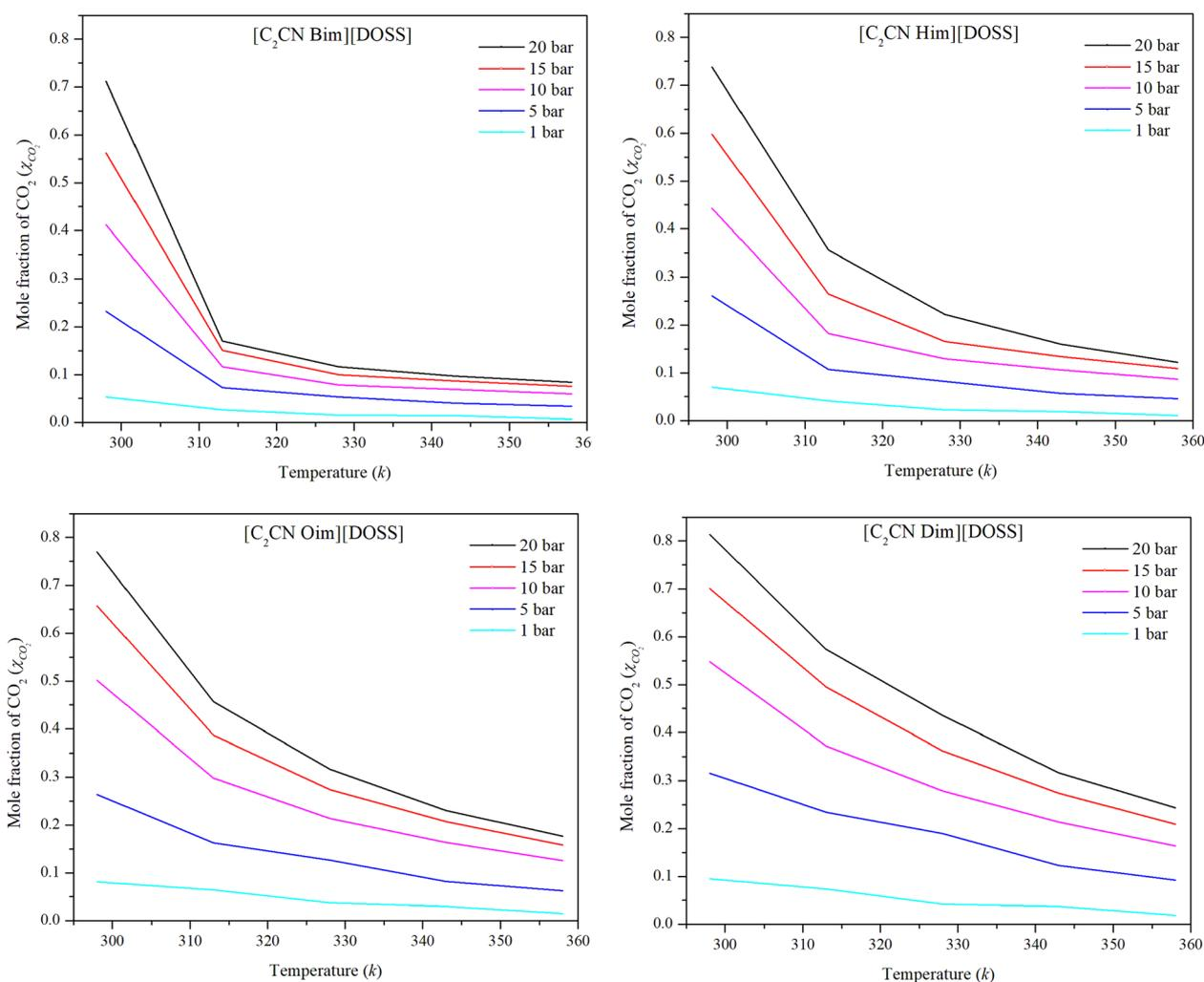
**Fig. 5** Experimental data on the solubility of CO<sub>2</sub> in [DOSS]-based ILs at various temperatures and pressures.
