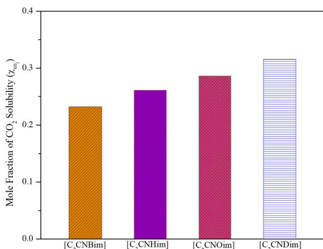
Fig. 3 Effect of cations on CO<sub>2</sub> solubility in the synthesized ILs at a temperature of 278.15 K and a pressure of 5 bar.
