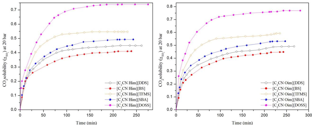
Fig. 2 CO<sub>2</sub> solubility in the [C<sub>2</sub>CN Him] and [C<sub>2</sub>CN Oim]-based ILs incorporated with [DDS], [BS], [TFMS], [SBA] and [DOSS] anions at 298.15 K at 20 bar.
