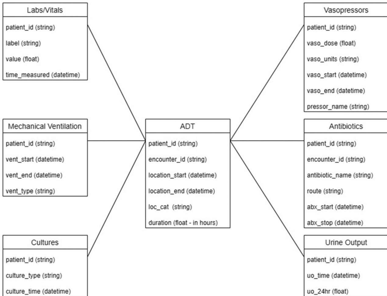
Figure 1. Minimal Sepsis Data Model. Dataframes needed by the python pipeline to determine Sepsis-3 onset.
