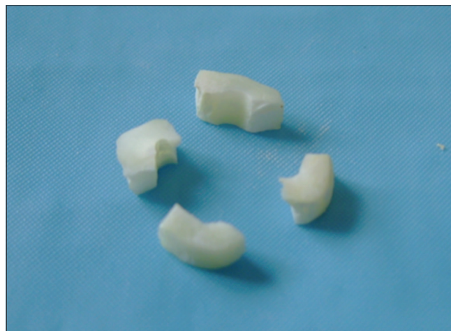
Figure 2: Slice sectioned in four equal sections, obtaining a total of four (S1, S2, S3, S4) samples
