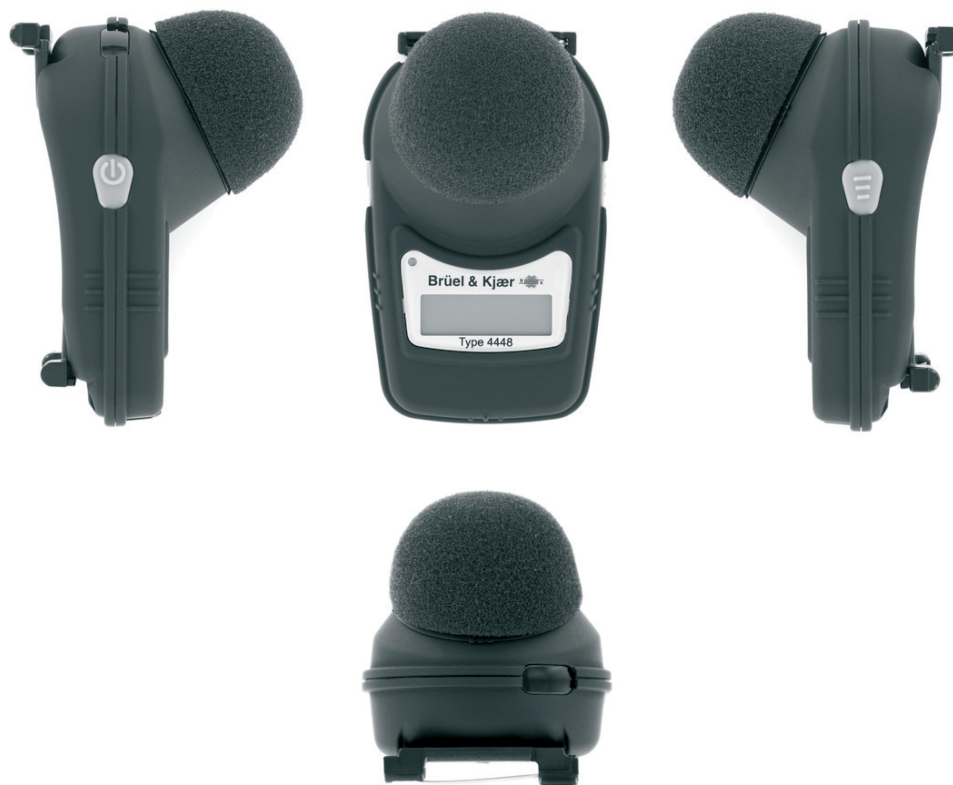
Figure 2 Personal dosimeter type 4448 (Denmark brand) used for aerial noise level measurement.
