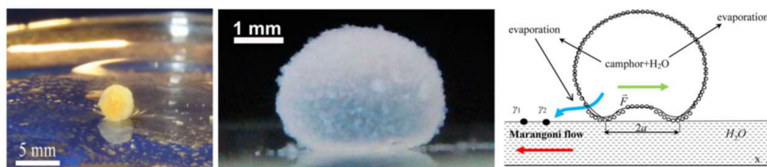
Figure 24. Self-propulsion microfluidic system inspired by chemotaxis for the manipulation of marbles on water. The left figure shows a marble filled with camphor, and the right figure shows a sample physical configuration of the problem. Reprinted with permission from [165]. The middle figure shows a moving marble containing 70% ethanol. Reprinted with permission from [166].
