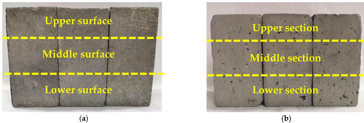
Figure 3. Diagram of the different test areas for the nominal strength of the sample: (a) the surface of the sample; (b) the cutting surface of the sample.
