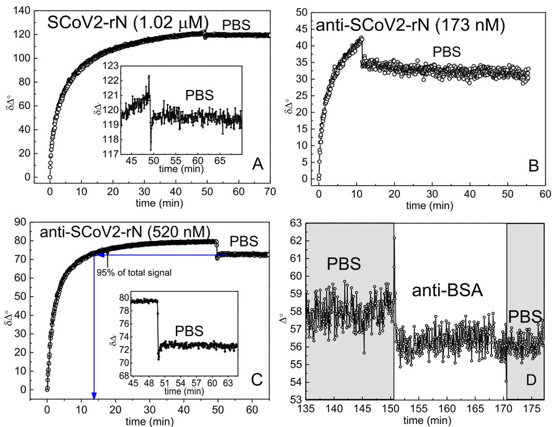
**Fig. 2.** Time resolved TIRE signals registered for: Immobilization of SCoV2-rN on Au/11-MUA activated by EDC/NHS (A). **Inset in A** – Au/11-MUA/SCoV2-rN washing at the time interval from 49 min to 70 min. Affinity interaction of anti-SCoV2-rN using 173 nM (B) and 520 nM (C) concentration with SCoV2-rN immobilized on the surface. **Inset in C** – the dissociation phase of the immune complexes. Nonspecific interaction of Au/11-MUA/SCoV2-rN structure with anti-BSA antibodies (D).
