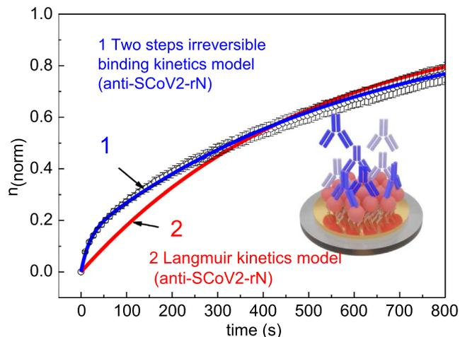
**Fig. 6.** Results of different kinetics analysis models applied for SCoV2-rN/anti-SCoV2-rN complex formation (Au/11-MUA/SCoV2-rN/anti-SCoV2-rN): 1 - two steps based consecutive irreversible binding model, 2 - Langmuir model.
