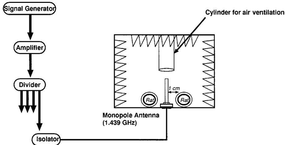
Fig. 1. Diagram of the exposure apparatus. Exposure conditions: frequency, 1.439 GHz; antenna input, 0.33 W (PDC modulation); animals, F344 male rats; duration, 90 min/day, 5 days/week, 6 weeks.
