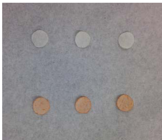
Figure 1 Light image of selenium coated and uncoated paper towels. Notes: The three pieces on the top are paper towels without selenium coating. The three on the bottom are paper towels coated with selenium nanoparticles. The diameter of each sample equals to 7 mm.
