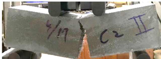
Figure 4. Failure of the experimental group specimen in flexure test.
