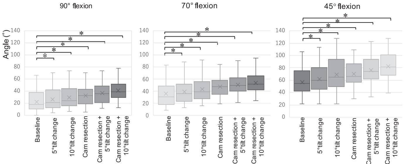
**Figure 3.** Maximum internal rotation at 45°, 70°, and 90° of flexion for the pelvic tilt change, cam resection, and combined models. In all 3 flexion conditions, the combination of a cam resection with a 10° pelvic tilt change showed the largest internal rotation. The shadow boxes indicate the interquartile range, the middle line indicates the median, the X indicates the mean, and the whiskers indicate the range. \* $P < .001$  compared with baseline.
