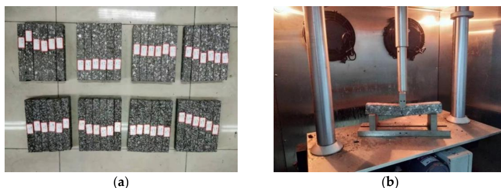
Figure 3. Low temperature trabecular bending test: (a) forming trabecular specimen; (b) test photo.
