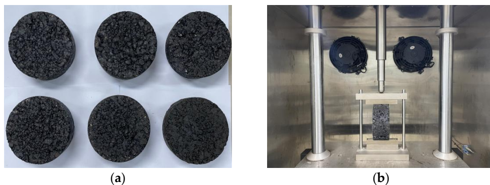
Figure 5. IDEAL cracking test: (a) forming trabecular specimen; (b) test photo.
