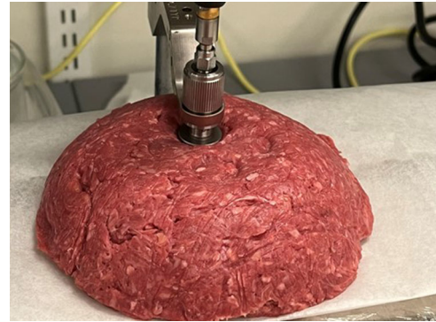
FIGURE 2 | Dielectric probe in contact with ground beef sample during measurement.
