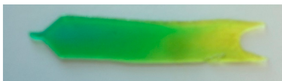
Figure 1. Demonstration of colorimetric gradient in a polyethylene glycol hydrogel. Adapted with the permission from [73]. Copyright 2015 Elsevier.
