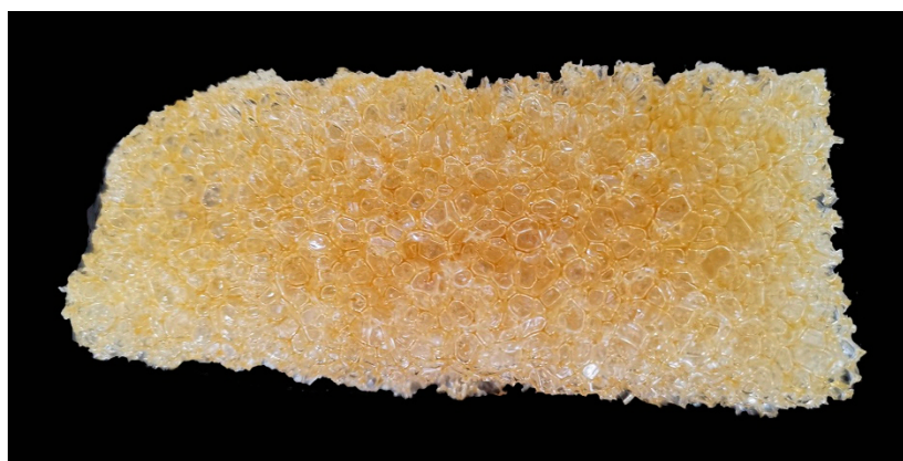
Figure 11. Cross-sectional view of polyurethane foams prepared using liquefied products at 110 min liquefaction time.
