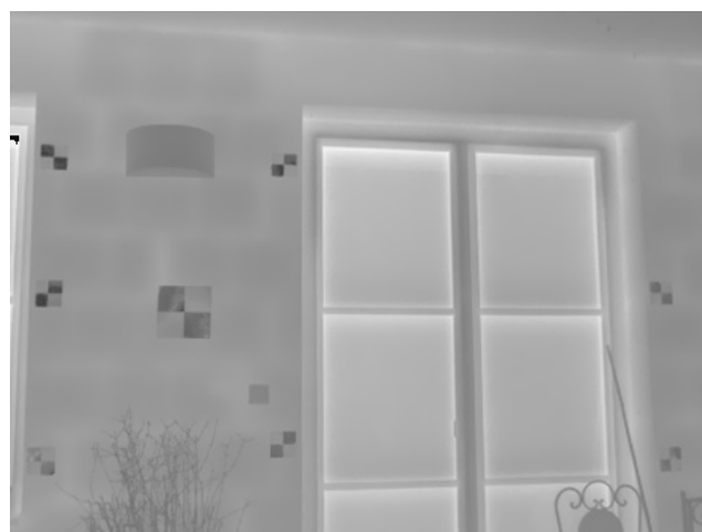
Figure 4. Image captured from 4 m distance. In the image are recognizable cross aluminum paper targets.
