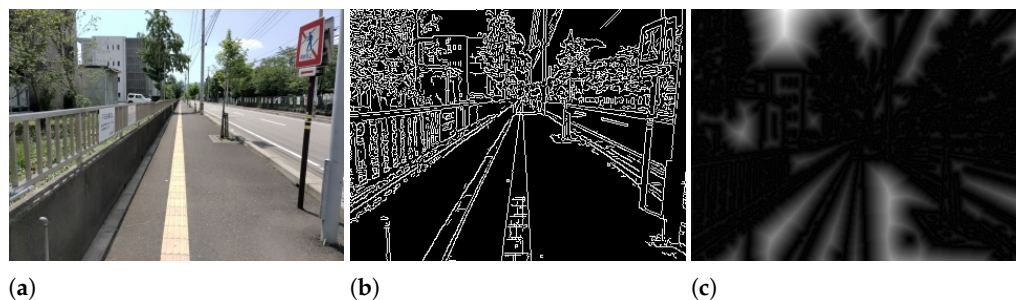
Figure 5. (a) Input image, (b) Edge image, (c) Distance transform image.
