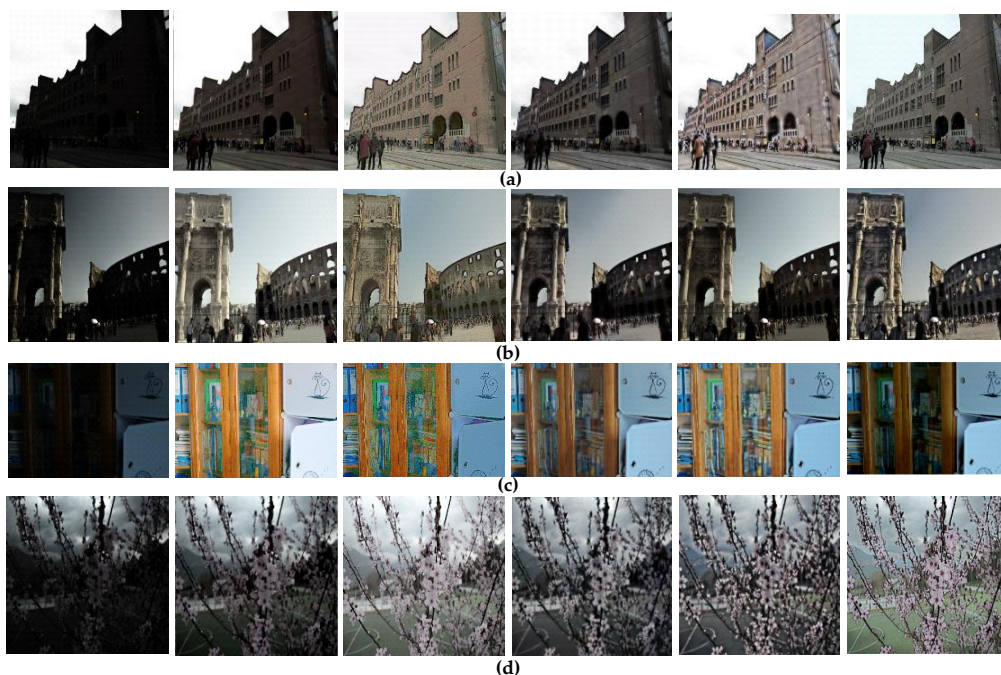
Figure 6. Low-illumination MSRCR RetinexNet KinD MBLEN Ours. Comparison of the processing effects on the general dataset. the leftmost column is the low-illumination image, and the other four columns are the results of the low-illumination image processed by MSRCR, RetinexNet, KinD, MBLEN and our proposed algorithms.
