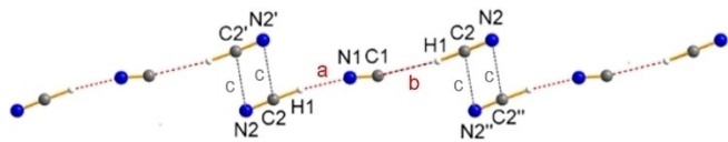
Figure 2. Ball-and-stick representation of a section of [\text{CN}(\text{HCN})_2]^- anion strands in the crystal of [\text{Ph}_4\text{P}][\text{CN}(\text{HCN})_2] . Red dashed lines (a and b) show hydrogen bonding whereas the grey dashed lines (c) show weak Van der Waals interactions.
