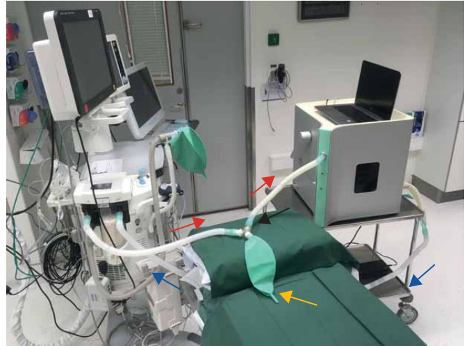
FIGURE 3 The respiratory circuit. The yellow arrow shows the balloon representing the patient and the black arrow, the non-rebreathing valve. The red arrows shows the direction of airflow from the mechanical ventilator to the balloon representing the patient and further on to the particles in exhaled air (PExA) device. The blue arrows show the direction of airflow from the PExA device back to the ventilator.
