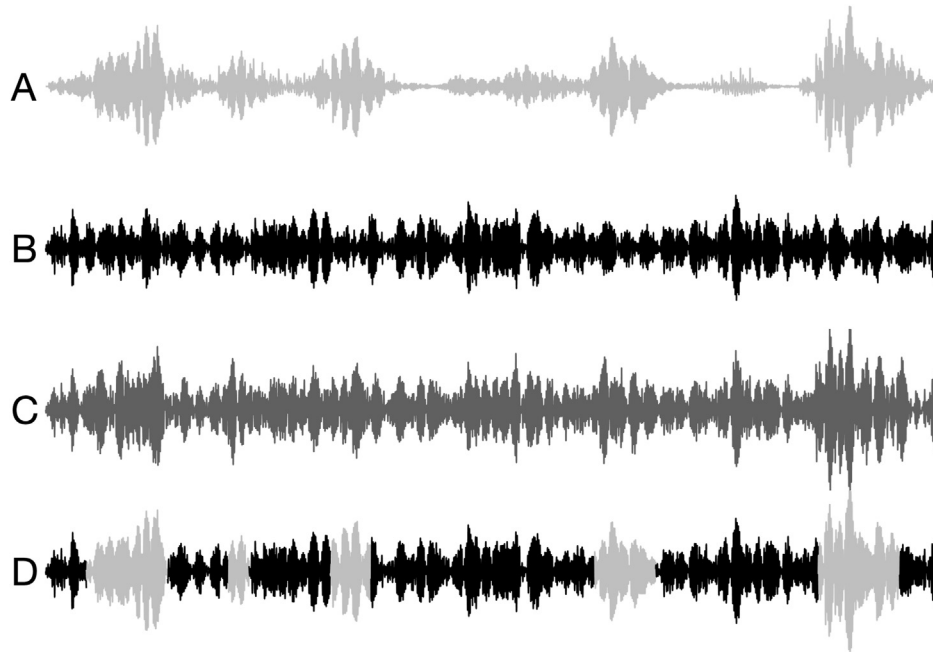
Fig. 2. Illustration of the “winner-takes-all” mechanism for energetic masking. A: Waveform of the first 884 msec of a Mandarin AzBio sentence (List F Sentence 15) (Xu et al., 2020) passed through a bandpass filter between 801 and 925 Hz. This band was approximately 1 ERB wide (Stone et al., 2012). B: Waveform of an 884-msec long speech-spectrum-shaped noise passed through the same bandpass filter. The amplitude of the noise was adjusted so that the root-mean-squared value was equal to that of the speech signal, thus the signal-to-noise ratio was 0 dB. C: Speech in noise (i.e., A + B). D: The “winner-takes-all” result. A time bin was set at 20 ms (Brungart et al., 2006). For all time bins in which the speech amplitude was greater than the noise amplitude, the speech waveform was plotted in light gray. Otherwise, the noise waveform was plotted in black.
