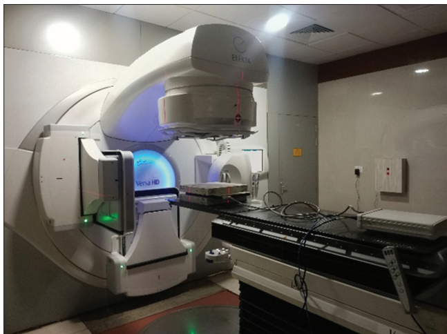
Figure 2: The patient-specific quality assurance setup in the linac bunker
