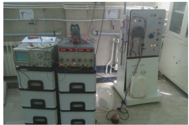
Figure 4. Modification of the First Circuit Using Expired Blood
