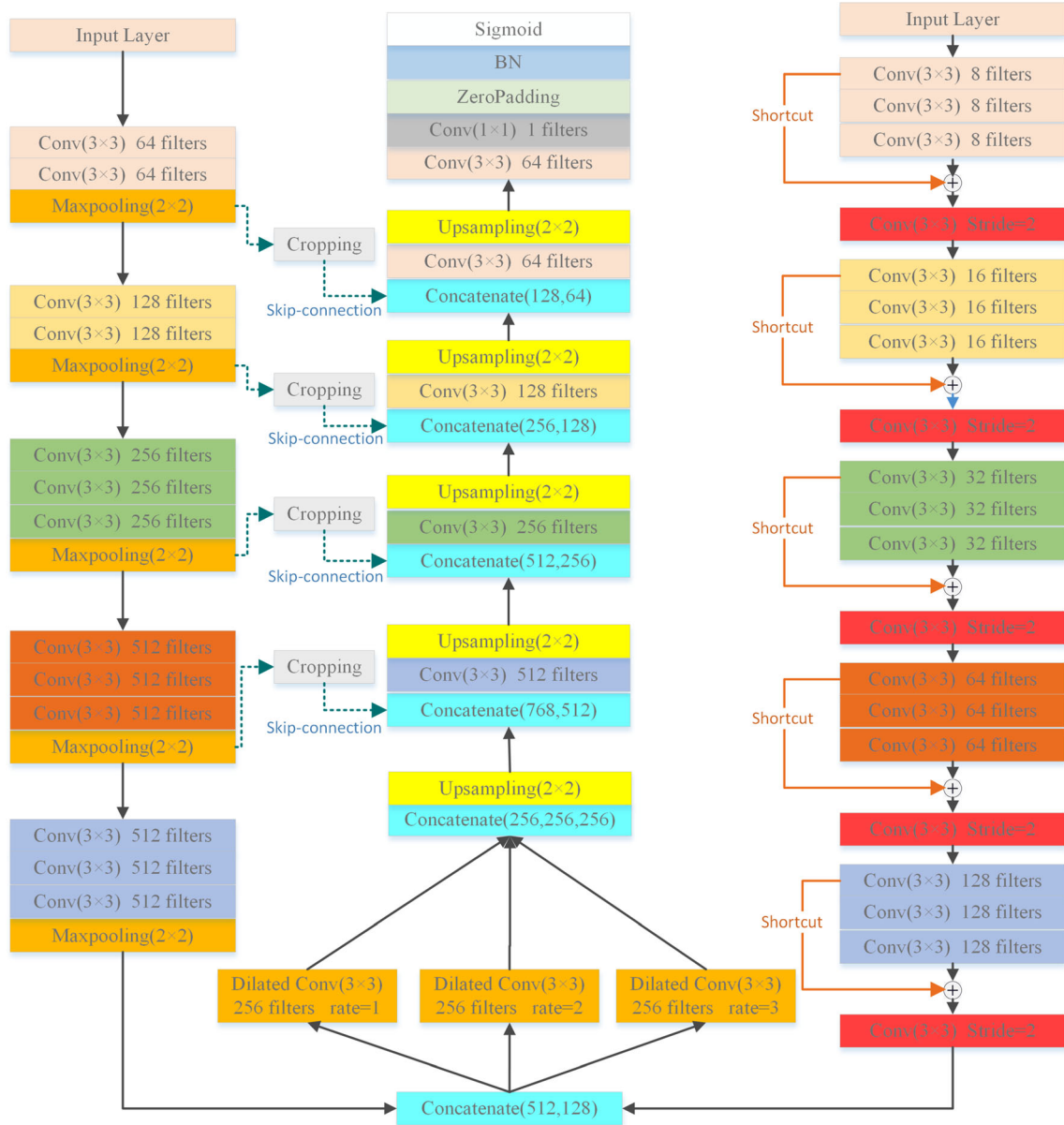
Fig. 4 DCU-Net model structure for image splicing forgery detection. There are two encoders on the left and right sides. The input is tampered image and residual image. At the bottom is the feature fusion module, the first is the fusion of image features and residual
