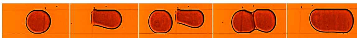
Figure 6. Sequence of trapping, fusion, and detachment of slug droplets over a narrow band of GO. The dimensions of the channel ( W \times H ) are 200 \mu\text{m} \times 50 \mu\text{m} . The width of the GO pattern is approximately 10 \mu\text{m} and is patterned along the width of the channel.
