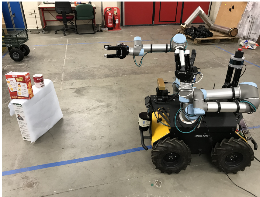
Figure 10. Clearpath dual UR5 arm Husky robot used for the real-world experiments.
