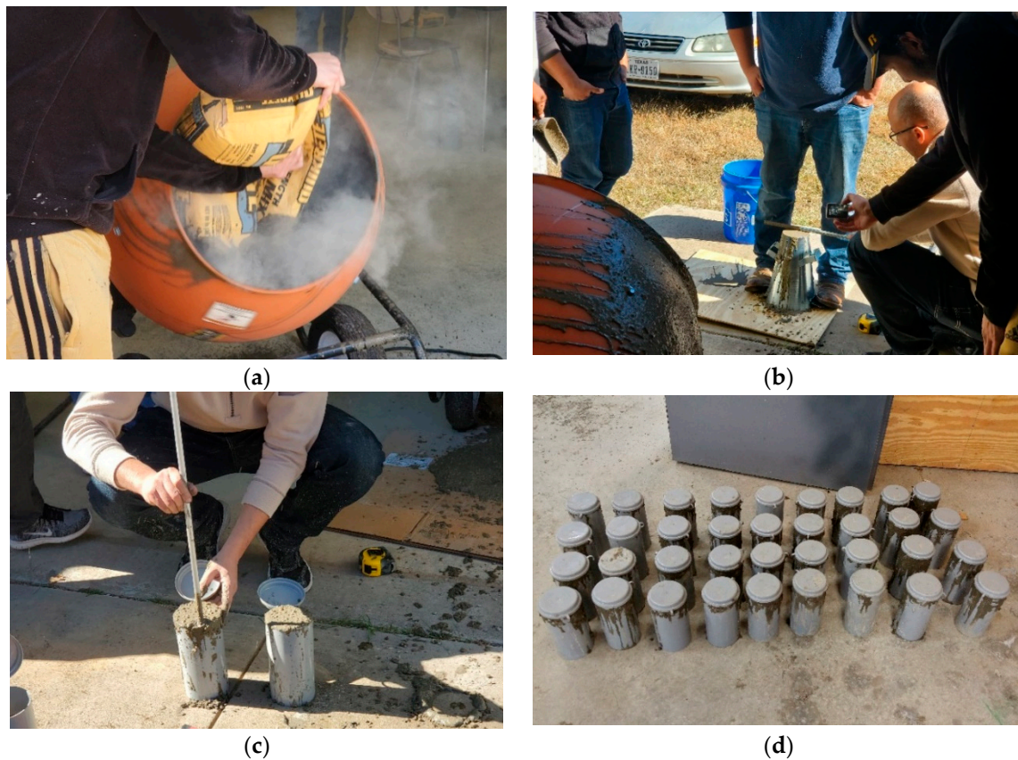
Figure 2. Preparation process of the concrete cylinders: (a) mixing concrete; (b) slump test; (c) pouring concrete; (d) concrete specimens in plastic molds.
