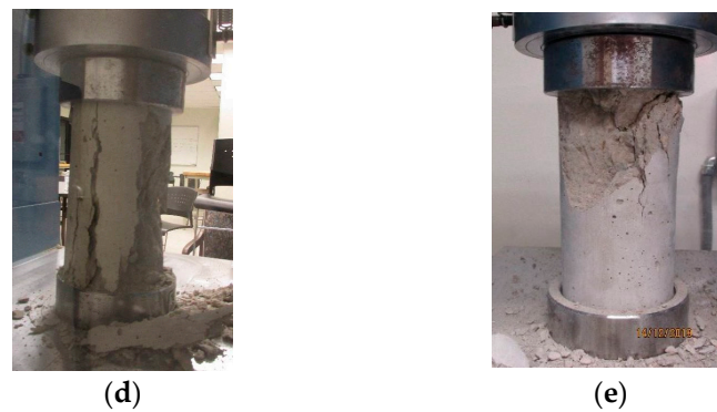
Figure 7. Modes of failure at age of 28 days: (a) T = 0\text{ }^{\circ}\text{C} (well-formed cone and vertical cracks); (b) T = 21\text{ }^{\circ}\text{C} (well-formed cone); (c) T = 40\text{ }^{\circ}\text{C} (well-formed cone); (d) T = 121\text{ }^{\circ}\text{C} (columnar vertical cracking); (e) T = 260\text{ }^{\circ}\text{C} (side fractures at top).
