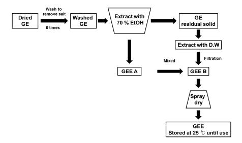
Figure 2. Preparation procedure for GEE [10].
