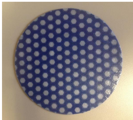
Figure 7. Final viscoelastic layers combining 3D printing and spin coating layers.
