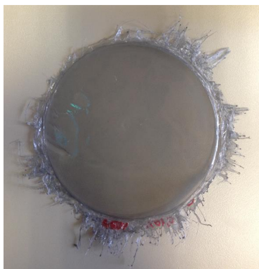
Figure 5. Multilayer film created by spin coating, composed of 3 reinforced ABS layers reinforced with 0.10%, 0.25%, and 0.50% CNS, respectively.
