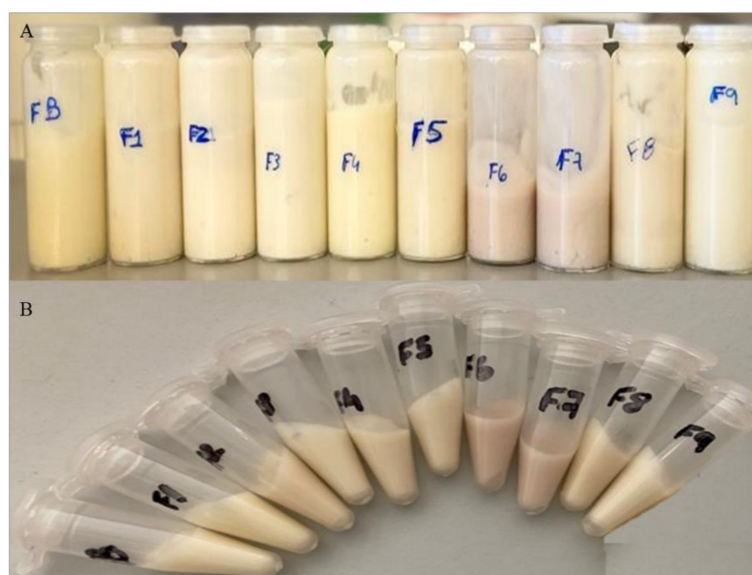
Figure 3. Face creams appearance after thermal stability test (A) and centrifugation test (B).
