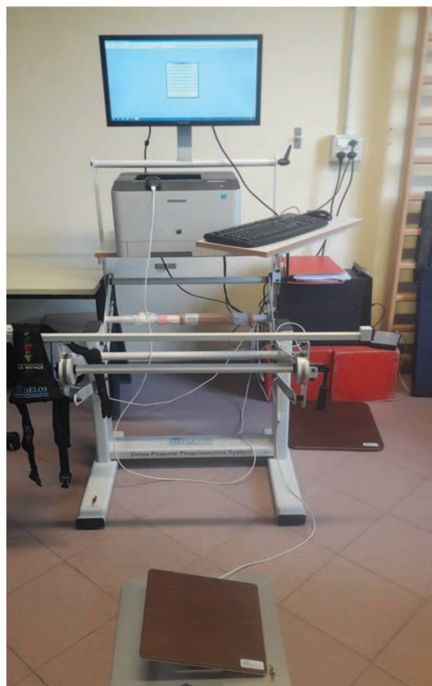
Figure 2. The DELOS Postural Proprioceptive System (DELOSs.r.l., Turin, Italy) was used for this study. The horizontal bar, the Delos Assistant Desk (DAD), fitted with an infra-red sensor, is set in front of the patient for hand support. The DAD measures the times and the duration of leaning the hands of the patient, expresses in terms of percentage providing information about the so called “precautionary strategy” that is the way the patients prevent falls, and regain the vertical posture.
