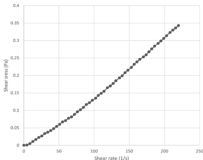
**Figure 2.** Flow curve a shear stress/shear rate of citronella nanoemulsion.
