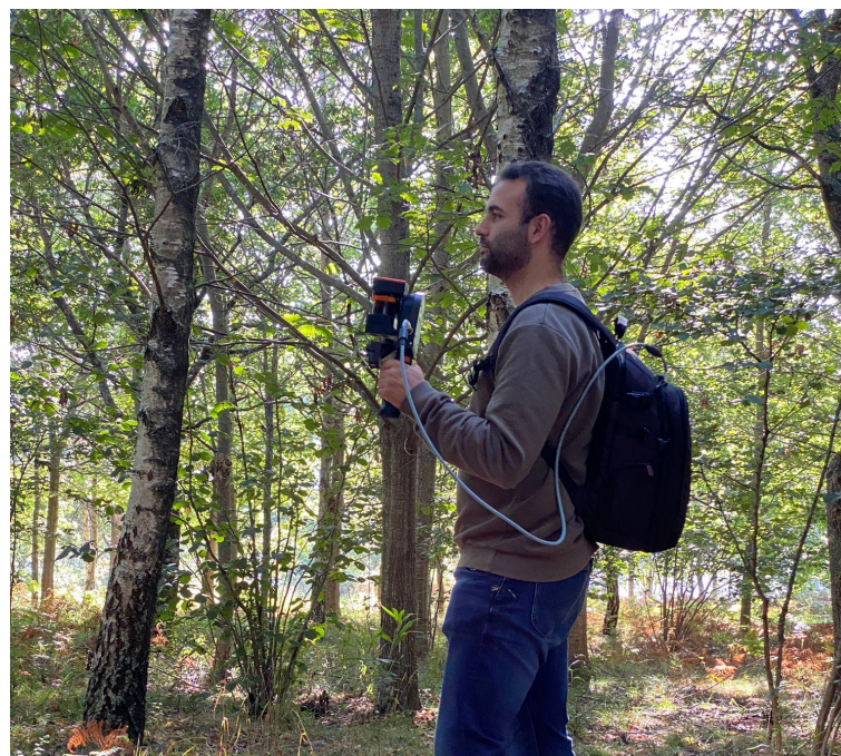
Figure 1. Backpack LiDAR system used during the data acquisition in the study area.
