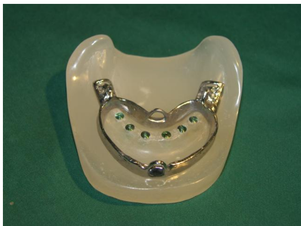
Fig 2. The framework with a special design seated on the test cast while encircling the six implants
