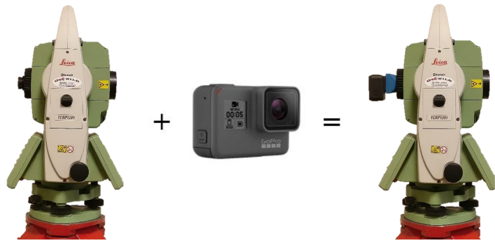
Figure 1. IATS prototype: Leica TPS1201 plus GoPro Hero5 camera.
