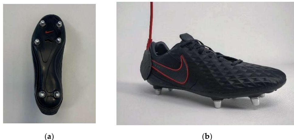
Figure 2. (a) Football shoe with six instrumented studs in the transversal plane (b) and integrated electronics at the back.
