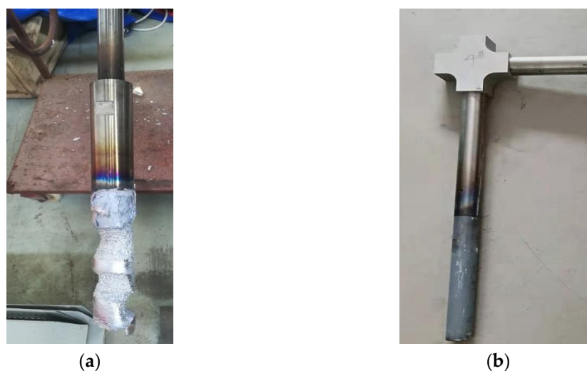
Figure 4. Morphology of sonotrodes: (a) straight-rod titanium alloy sonotrode; (b) L-shaped ceramic sonotrode.
